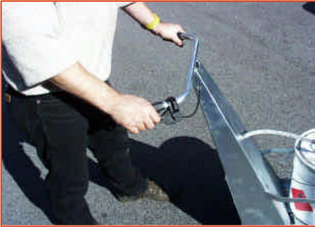
**Fig 6:** To spray pull handle grip. Releasing grip stops pump.
