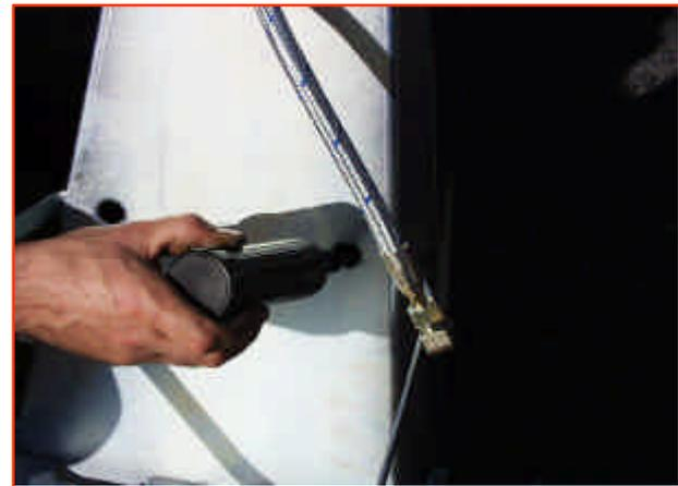
**Fig 9:** Grease pump at two grease points after intensive use.
